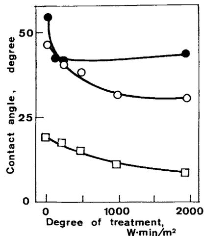
**Figure 3** Effect of degree of corona treatment of veneer (○) before and (□) after extraction with alcohol-benzene and (●) its extractives from Japanese red pine on their contact angle.
