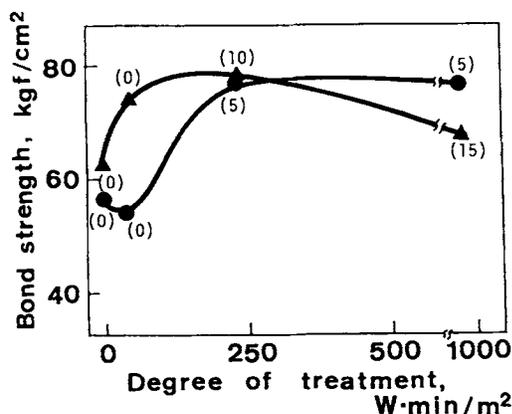
**Figure 4** Variation of bond strength with degree of corona treatment. The values in parentheses are wood failure: (●) isunoki; (▲) purpleheart.
