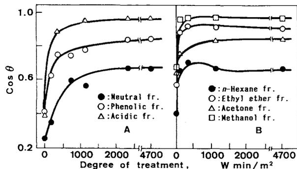
**Figure 5** Effect of the corona treatment of various fractions of extractives from Japanese red pine on their wettability: (A) fractionation method; (B) successive method.
