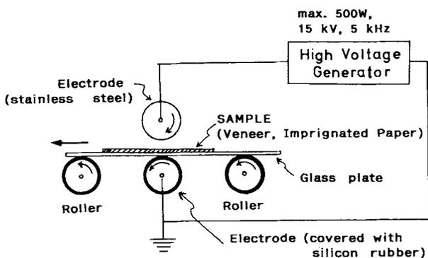
Figure 1 Diagram of corona-treatment apparatus.
