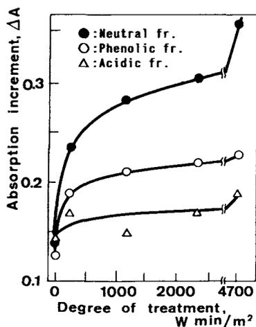
**Figure 6** Relation between the degree of treatment for the fractionated extractives from Japanese red pine and the absorption increment ( $\Delta A$ ) dyed with Schiff's reagent.
