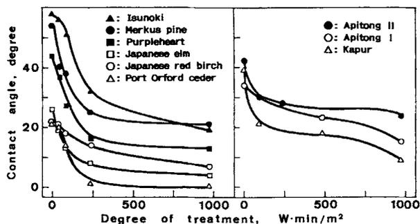
**Figure 2** Variation of contact angle for the veneers with degree of corona treatment.
